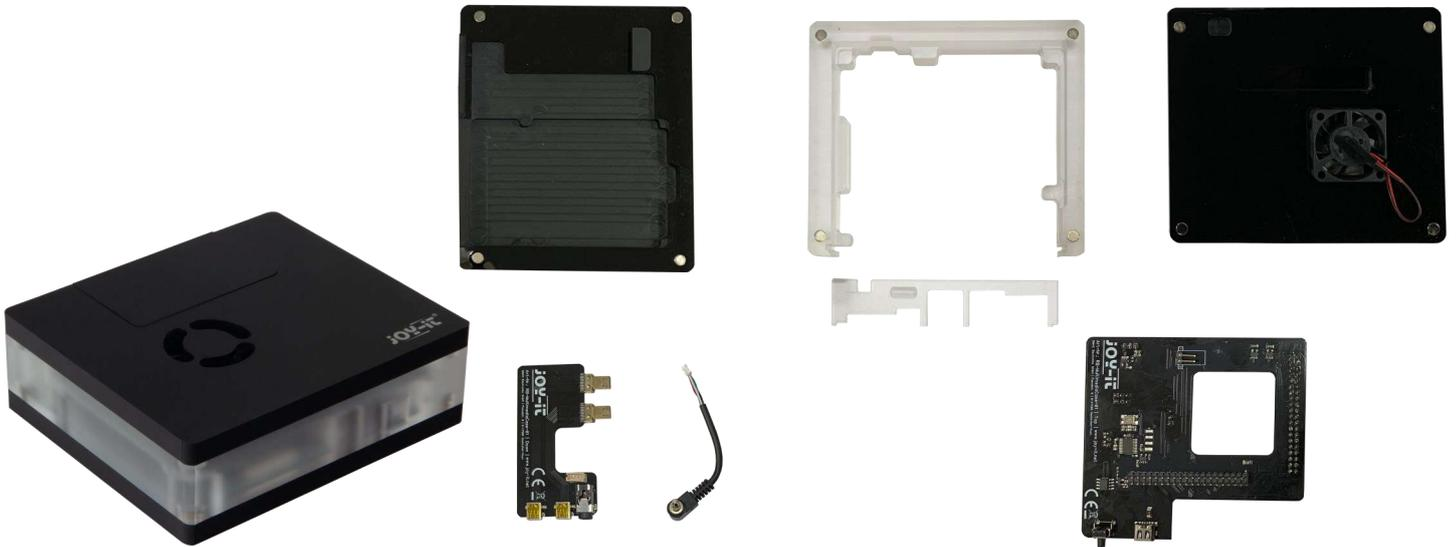
2. Then connect the AUX plug to the jack socket from the Raspberry Pi. Now insert the already written SD card into the Raspberry Pi. You find more information about that in **Chapter 2: Software installation**. Also attach the heat sink to the CPU of the Raspberry Pi.
